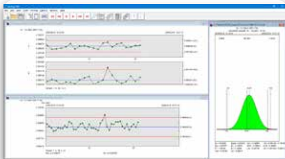
Statistical Process Control - Typical screen
