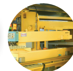
6 RM 210 CM X-ray Strip Thickness Gauge
